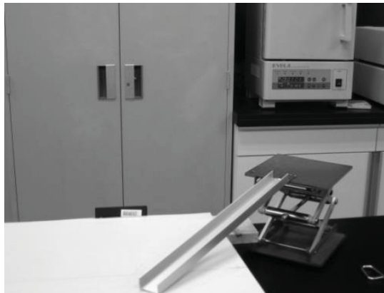
Figure 6. Laboratory Jack and Channel
